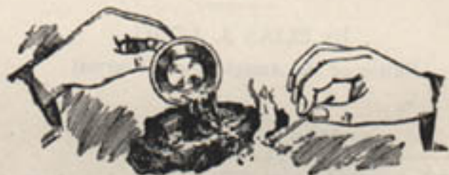
THE INSTANT WATER TOUCHES THE CARBIDE, CRUDE GAS ARISES READY FOR MATCH.
